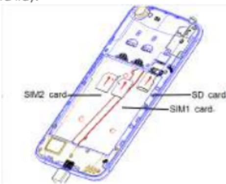
2. Locate the SIM card slot and insert the proper SIM card into the proper slot. For more information on SIM card installation, check out the included [SIM Card & Micro SD Card Installation Guide](#).
