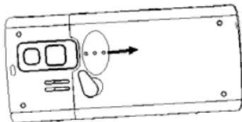
Close the case by locating the plastic cover into the grooves and *sliding* the cover up to close it. Do NOT force the cover down by pressing on it. This will damage the cover. Slide the cover up gently
