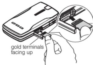
**Note** *Be sure to use only recommended microSD cards (64MB-8GB). Using non-recommended microSD cards could cause data loss and damage your phone.*
