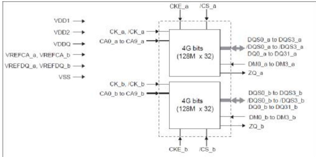
Figure 2-3 shows the model of the POP LPDDR2 chip provided by ELPIDA.
