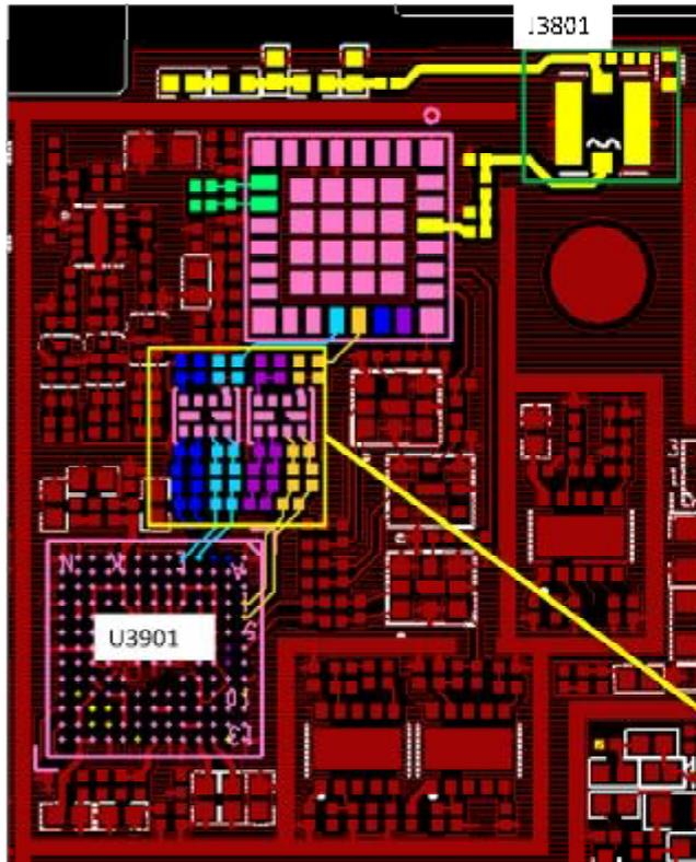
**Transmit:** The two green channels are transmit signals of the low-band GSM850/GSM900 and high-band DCS1800/PCS1900. They reach the RF connector 3801 after passing the GSM PA and the antenna switch U4101. The yellow parts indicate components on the channels of signals output by the antenna switch.
