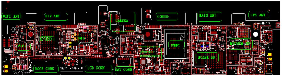
Figure 4-3 shows the physical architecture of the PCBA, where the interface connections of various modules are indicated. The application processor Hi3620 has three MIPI interfaces. The CSI interface is connected to the LCD module. The CSI0 interface is connected to the rear camera. The rest MIPI interface is a multiplexing of DSI and CSI to provide digital connections for the front camera.
