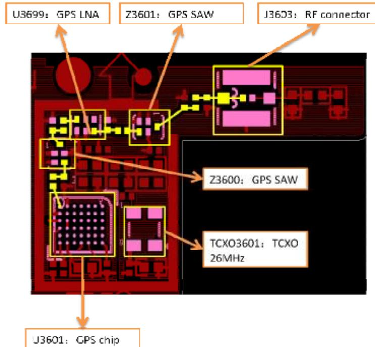
Yellow indicates GPS receive channels. GPS signals arrive at the GPS SAW filter Z3601 from the RF connector J3603. Then the signals are amplified by the LNA U3699, pass the GPS SAW filter Z3600, and finally reach the GPS chip.
