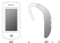
In the example illustrated above, if a hearing aid meets the M2 level rating and the wireless phone meets the M3 level rating, the sum of the two values equal M5. This should provide the hearing-aid user with “normal usage” while using their hearing aid with the particular wireless phone. “Normal usage” in this context is defined as a signal quality that’s acceptable for normal operation.
