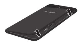
Press along the edge of the back cover until you have a secure seal.
