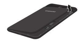
**Caution**: When removing the back cover, use the slot next to the Volume key to gently lift the cover off. Pulling on the Speaker (located next to the Power key) may cause damage.
