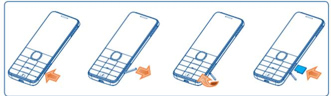
Insert the microSD card with the golden contact upward. To remove the card, press and slide it out.
