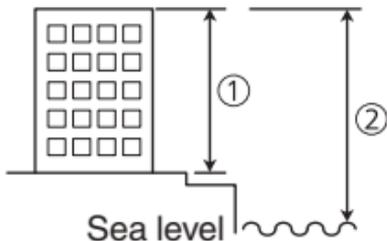
Your watch's Altimeter use a pressure sensor to measure barometric pressure, and then calculates and displays relative altitude based on the measured value. The altitude values displayed by your watch are based on International Standard Atmosphere (ISA) relative altitude data defined by the International Civil Aviation Organization (ICAO).
