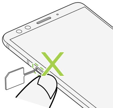
3. Push the tip all the way into the hole until the tray ejects, and then pull the tray out.
