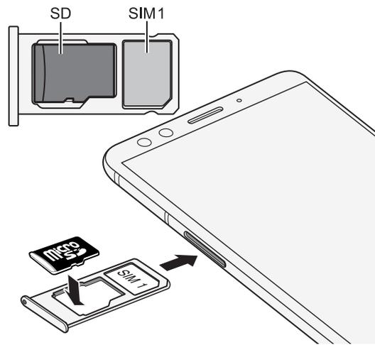
5. When reinserting the tray, make sure it is facing up so that your cards don't fall out. With the outer card holder between your fingers, steadily slide the tray all the way into the slot.
