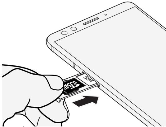
6. Make sure the tray is fully inserted and doesn't protrude from the slot.
